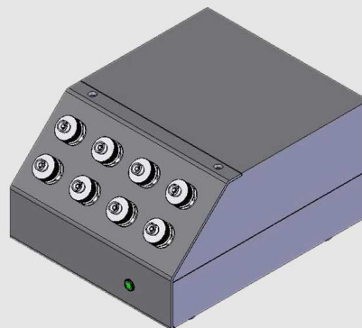
8 Channel Power Meter
